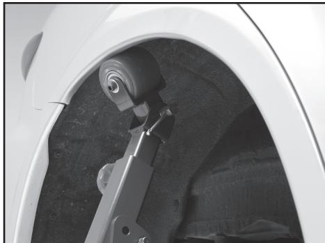
**Step 7:** Continue rolling and adjusting your roller head by increasing the angle. You are slowly working the lip up flush with the inner surface of the fender arch.
