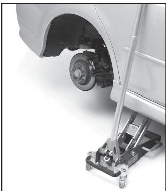
**Step 2:** Remove the tire/wheel and set aside.
