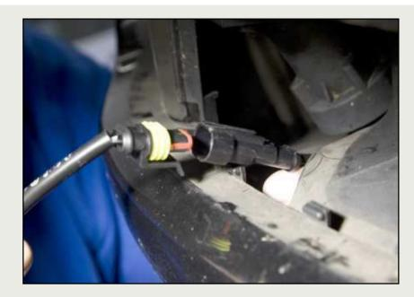
Once the LED modules have been mounted, the lights only have to be connected to the control units and then the covers inserted into the front apron.
