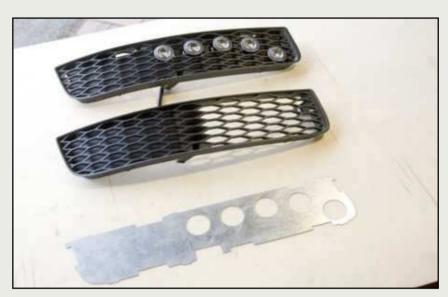
The individual LED modules now have to be mounted. The right and left-hand trims on the front bumper are suitable for this. Since the lights are part of a universal daytime running light set, the covers have to be utilized.
