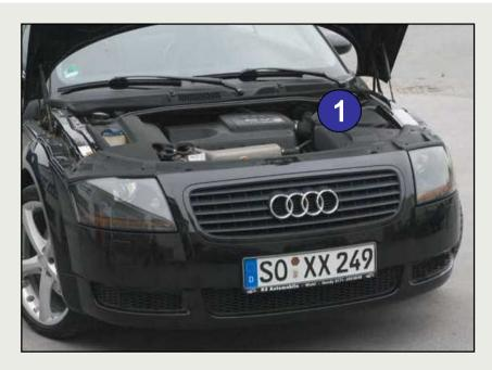
The cable has to be routed from the engine compartment to the interior first. This is possible at the point shown (1). Since the fuse box with terminal 15 is at the side of the dashboard in the Audi TT, the connection cable set is extended with the aid of the blue cable.
