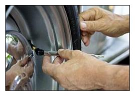
Step 3: If the tire pressure is too high in any of the tires, slowly release air by gently pressing on the tire valve stem so that you hear the air escaping until you get to the correct pressure.
