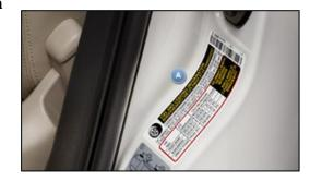
Step 2: Check the pressure of all tires, including your spare, using a tire pressure gauge. To check the inflation pressure of a tire, first unscrew the valve stem cap. Make sure that your pressure gauge is reset. To reset a standard stick gauge, push the stick with the pressure scale back into the casing. Now you're ready to check your pressure. Place your tire pressure gauge over the valve stem and press firmly to get a good fit. The tire's inflation pressure is measured by the pressure gauge.
