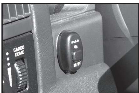
Suggested switch location. A round file should be used to allow the wire to go through plastic without pinching.
