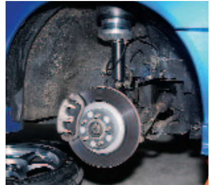
The struts mount like conventional struts, except for the air line and the wheel position sensor (on the right).
