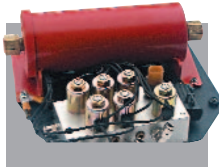
The valve block, hidden in the rear fender, takes commands from the Praxis ECU to distribute air pressure to each air spring. During the leveling process, the system automatically corner weights the car. The big red thing is a dryer to remove moisture from the compressed air.
