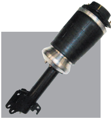
The strut comes completely pre-assembled, including the top mount, so there's no need for a spring compressor to remove the stock top mount. Also, note the tapered aluminum piston on the bottom responsible for the different spring rates in each mode.
