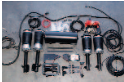
The kit is as complete as it is extensive. All this stuff adds 30 pounds to the car, but it's well hidden in various nooks and crannies, so the only visible parts are the switch to change ride height and the air tank in the trunk.
