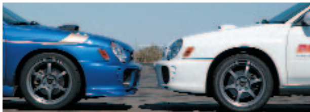
Touring mode is stock ride height, track mode is 2 inches lower. Changing them means pushing a button and twisting a knob under each strut.
